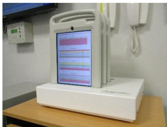
Tough-PAC® disguises iOS devices, provides protection against damage, is inherently anti-microbial and enables effective cleaning with infection control sprays or wipes without compromising the device.
