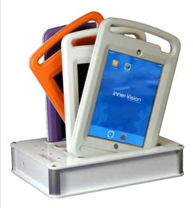
Tough-PAC's versatility as a mobile tablet PC is further enhanced by the Charge Station Management Consul. The CS4-MC allows charging or synchronising up to 4 Tough-PAC units simultaneously using 'Simply-Dock' interface technology.
